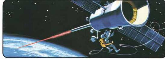
▲ This satellite, shown being serviced by an astronaut-engineer, has a laser to measure the small movements in the Earth's crust which are early indicators of earthquakes. This one is focused on a reflector embedded in the ground near the
