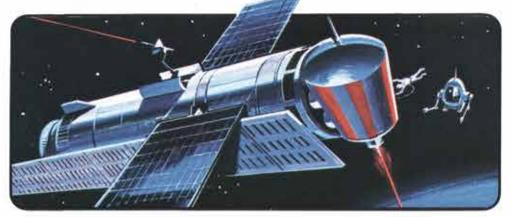
▲ This 14-tonne satellite, which could be in orbit by 1985, is designed to observe pollution and resources. It has two lasers one above the solar cell 'wings' for communication with other satellites; the other, pointed downwards, is used to check
