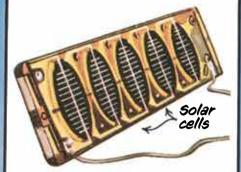
Solar cells are flat panes of silicon material which convert the energy in sunlight into electricity. A panel like this could help charge the car.
